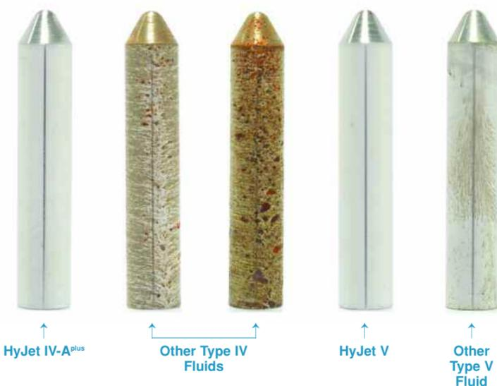
The ASTM D 665A test identifies rust on polished steel rods that have been exposed to 10 percent water in fluid for 24 hours at 60°C. HyJet V combats corrosion better than competitive Type IV and Type V hydraulic fluids.
